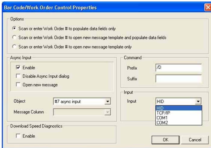
Figure 202 Bar Code Control and Properties
